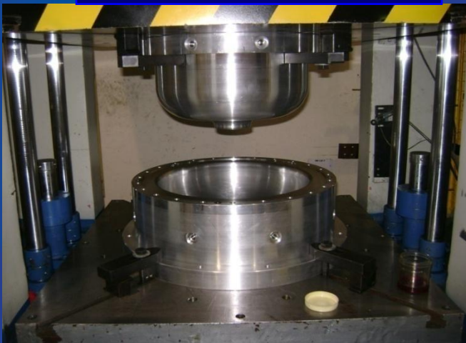
Die-Punch Set mounted on Press at RRCAT
